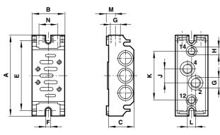
Side and Bottom Ports. Pilot ports on bottom.
